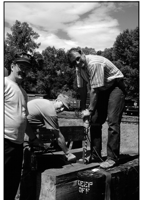
From left, Phil Scholl, Ken Gow and Steve Mason drilling the new pilot beam for RGS Engine #20. – Photo © Steve Mason
